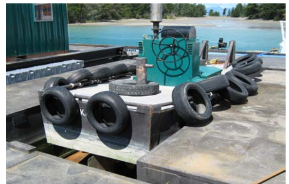
Below—The tug Kapai sits nicely in between a pair of the Kaimahi's pods. The two are ideally suited as both can be lifted out of the water and transportable via sea or land
